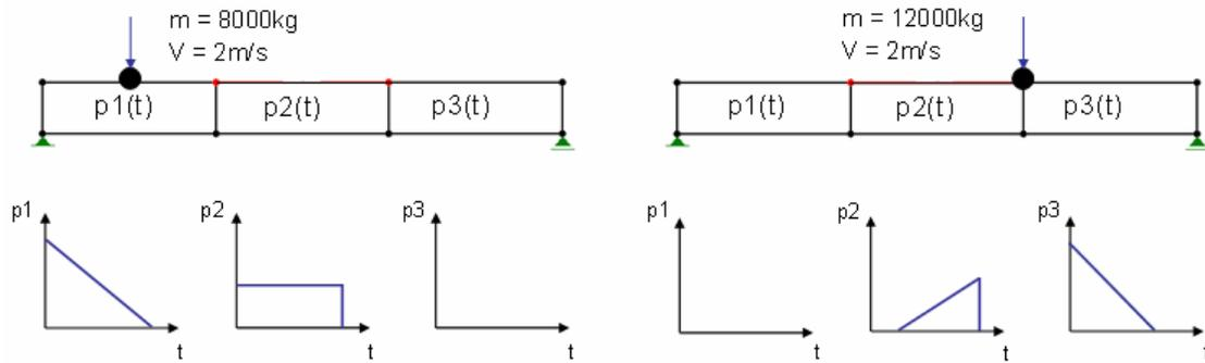
Figure 7: Strategy of the pressure distribution during lateral impact: a) over left chamber, b) over right partition
