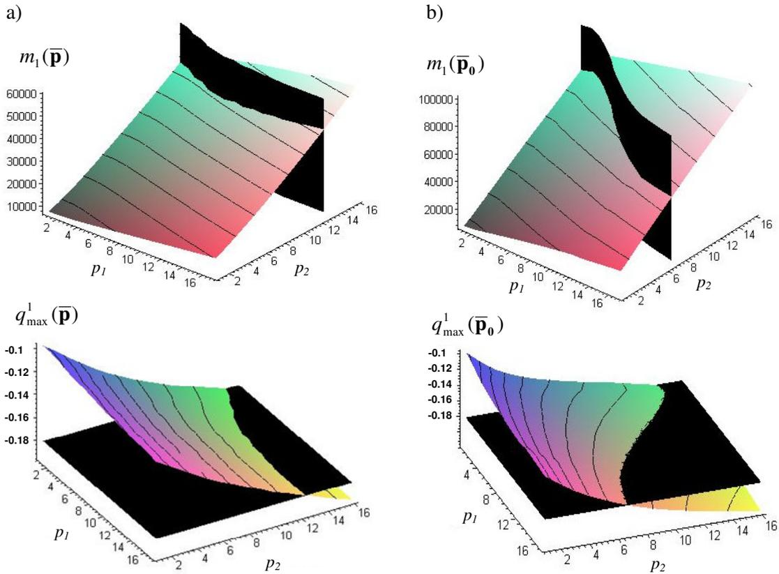
Figure 2: Surfaces  $m^1(\bar{\mathbf{p}})$  and  $q_{\max}^1(\bar{\mathbf{p}})$  in terms of non-dimensional pressure  $\bar{\mathbf{p}}$ , corresponding to the cases: a) constant value of pressure,  $\bar{\mathbf{p}} = \mathbf{p}/(100\text{kN/m})$ ; b) linear decrease of pressure,  $\bar{\mathbf{p}}_0 = \mathbf{p}_0/(300\text{kN/m})$ .
