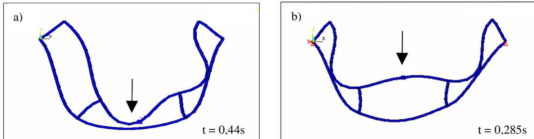
Figure 6: Deformation corresponding to fast (a) and slow (b) release of pressure in the middle cell.
