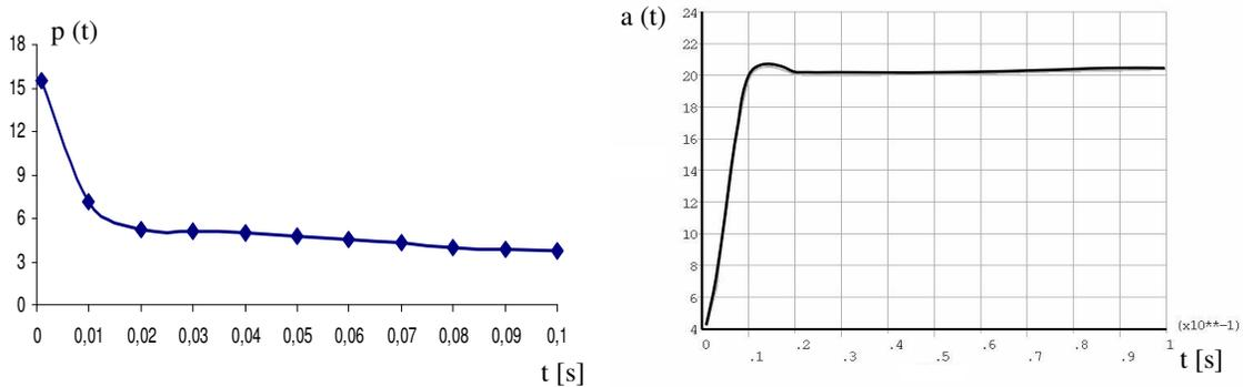
Figure 4: Results of the optimization: a) change of pressure in time; b) resulting acceleration of the hit joint
