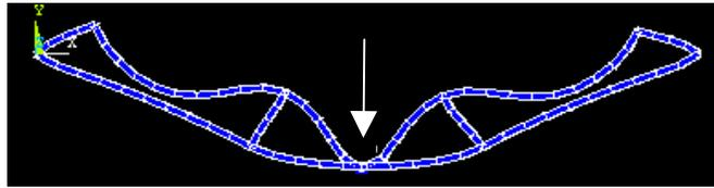
Figure 5: Desired deformation of the structure obtained by means of negative pressures
